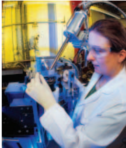
Installing a sample on a protein crystallography beamline at the Swiss Light Source.
